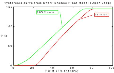
Figure 2. Hysteresis curve of plant model
