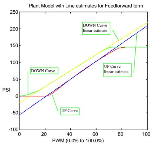
Figure 3. Plant Model with Line Estimates for Feedforward term
