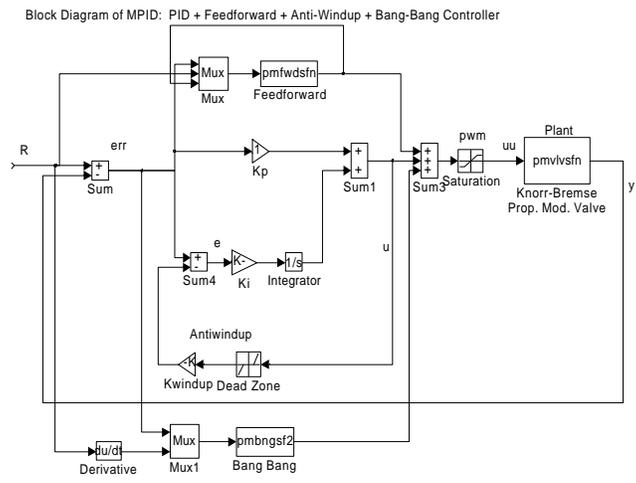
Figure 6. Block diagram of a MPID controller
