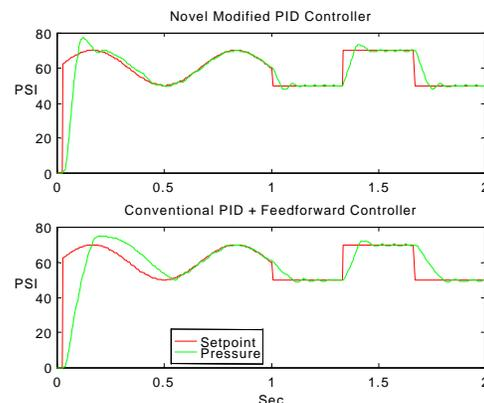
Figure 1. Comparison of MPID and Conventional PID
