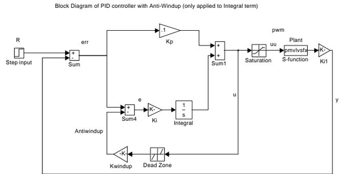
Figure 5. Block diagram of PID plus an Integrator Anti-Windup term
