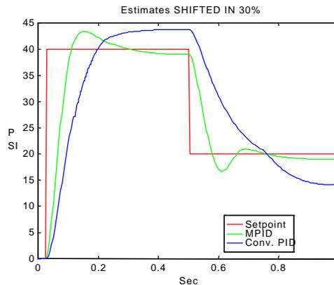
Figure 7. Comparison of conventional PID and MPID as the valve hysteresis varies by 30%
