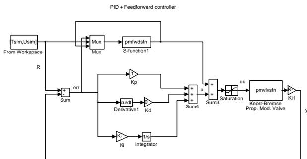
Figure 4. PID plus Feedforward block diagram
