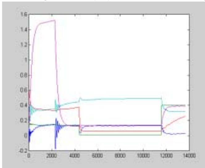
Figure 4. Parameter estimates for a sequence of different fault modes. The fault mode changes every 100 sec (at 0.05 sample/sec).
