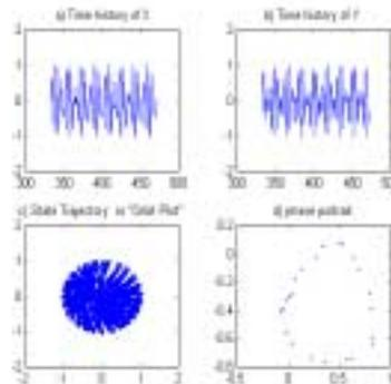
Figure 2. Time history, Orbit diagram and Poincare' map using [0.14, 1.33E3, 0.50, 0.49, 0.13].
