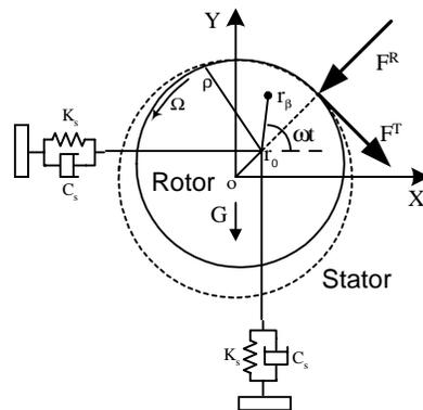
Figure 1. The rotor-stator interaction dynamics are modeled using a disk with 2-DOF within a circle.
