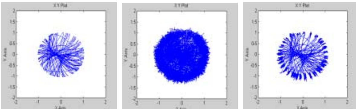
Figure 5. Orbit diagram for fault mode [200, 400] sec, of Figure 4. The predicted orbit of the rotor position (Right) is obtained from the simulated data (Middle) based on the estimated parameter. The Predicted orbit correlates to actual orbit (Left) except during transient time.
