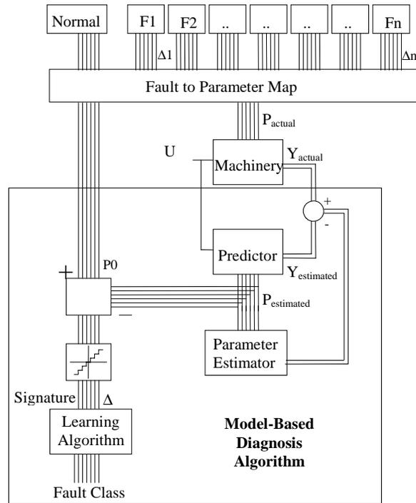
Figure 3. Block diagram of the proposed model-based diagnosis algorithm
