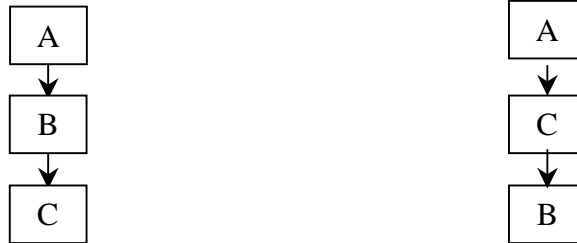
Before Processing After Processing Figure 3. Case I, page A has no free links, but C does.
