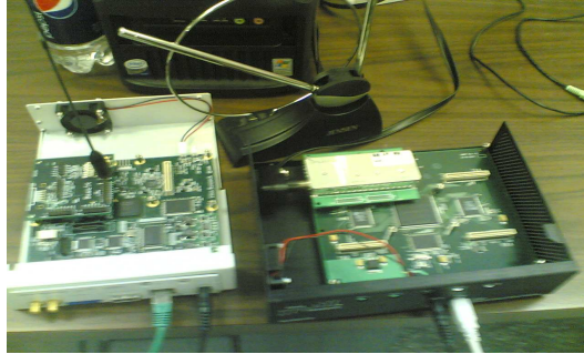
Figure 4 - Audio streaming over wireless channel from USRP2 to USRP1
