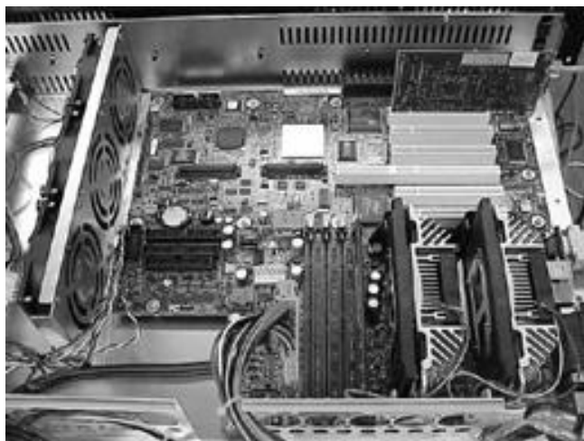
Inside of client board(Intel L440GX+)
