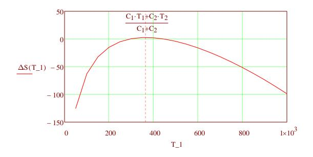
Note that at the equilibrium temperature:  $T_{MA} := \frac{C_1 \cdot T_1 + C_2 \cdot T_2}{C_1 + C_2}$ , T = 365.072 Kel vin $\Delta S$  the entropy increase is largest. Note that the entropy change for the object #1 (porcelain) is  $C_1 \cdot \ln\left(\frac{T}{T_1}\right) = 24.191$  calories/Kelvin and for object #2 (water) is  $C_2 \cdot \ln\left(\frac{T}{T_2}\right) = -21.484$  calories/Kelvin. The total entropy change is positive: 24.191 - 21.484 = 2.707 calories/Kelvin.
