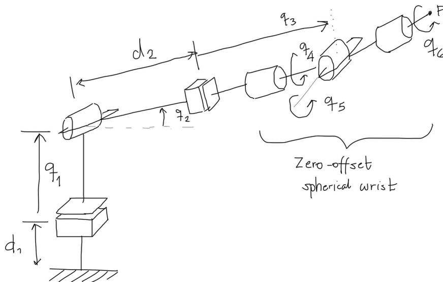
Figure 1: 6-dof robot with spherical wrist.
