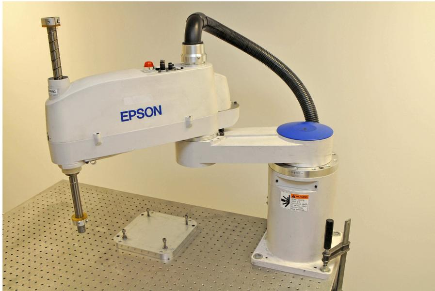
Figure 2: 4-dof SCARA robot.
