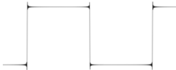
Figure 7.8: Illustration of Gibbs Phenomenon showing an “overshoot” near the jump discontinuities.
