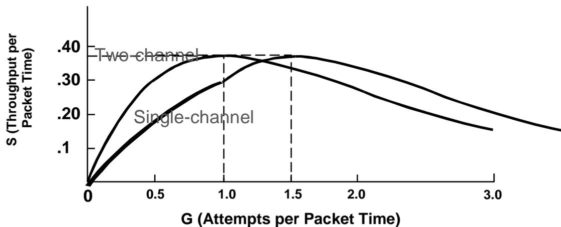
Figure 2: Performance comparison between two- and one-channel repeaters.
