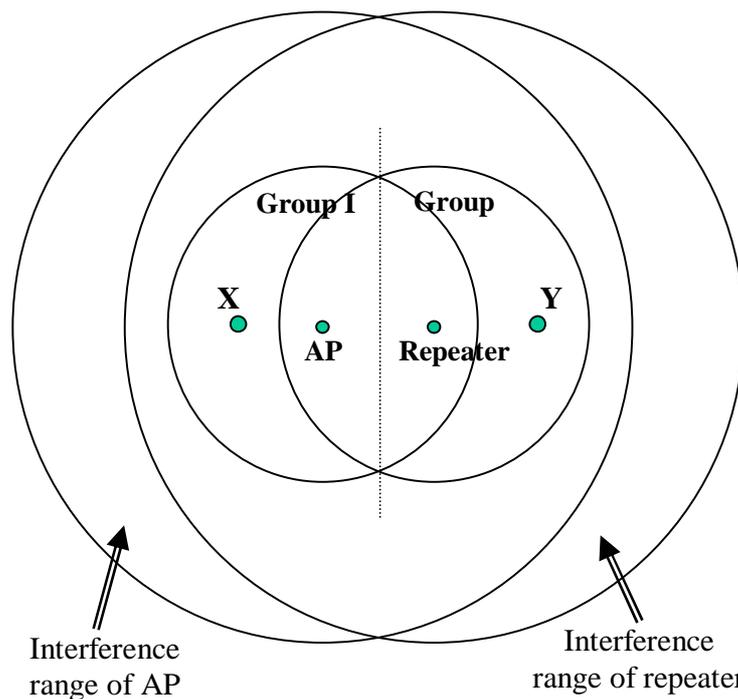
Figure 1: A simple mobile network with one AP and one RP.
