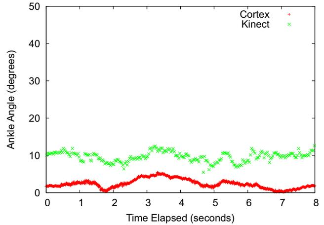
Fig. 7. Angle between the ankles and the frontal plane for a single iteration of sit to stand.
