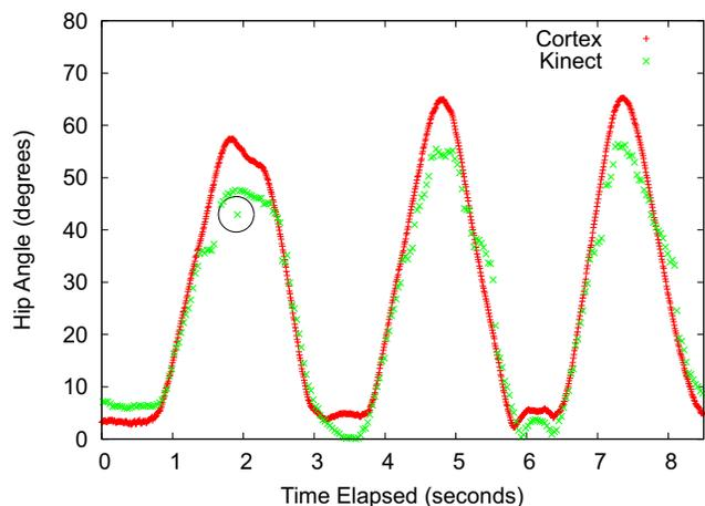
Fig. 1. Hip angle for 3 correct iterations of hip abduction.
