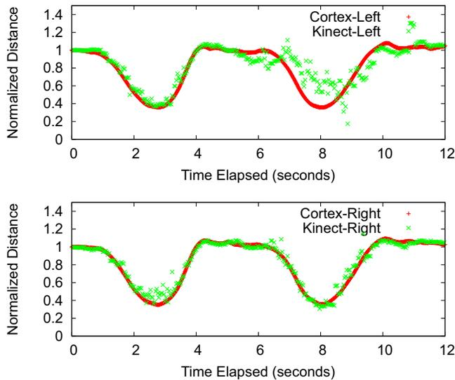
Fig. 10. Normalized wrist-to-ankle distance for 2 iterations in the toe touch exercise. The top figure is for the left side, and the bottom figure is for the right side
