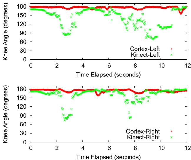
Fig. 11. Knee angle for 2 iterations in the toe touch exercise. The top figure is for the left knee, and the bottom figure is for the right knee.
